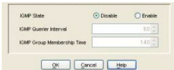
Figure 14-26. IGMP Setting for Routing Switches
